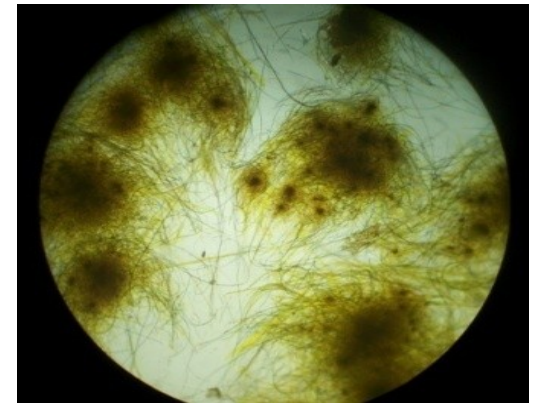
Powder puff/hedge hog shaped crystals of lactose as viewed under the microscope
